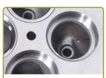
Machine all high-precision valve seat counterbores with one same cutting tool.
