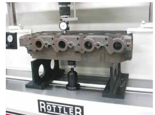
Rottler's small to medium diesel head fixture allows fast set up and clamping of in-line cylinder heads.
