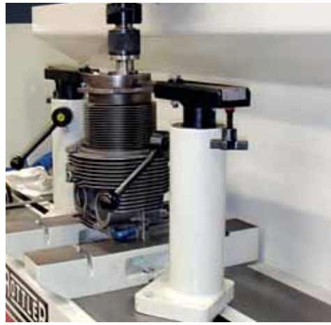
Rottler offers special fixturing for cutting seats in one piece aircraft cylinders.
