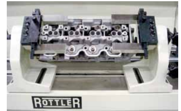
2 piece frame kit allows mounting of overhead camshaft and difficult to mount cylinder heads.
