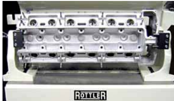
Rottler's 360 degree rollover fixture allows large, long heads, such as this Jaguar XJ6, to be rolled 360 degrees for multiple operations such as boring cam follow bores and repairing broken exhaust studs by drilling and tapping.
