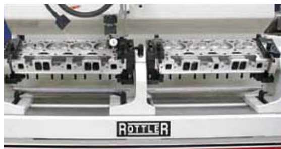
Dual Head Fixture allows a set of V6 or V8 heads to be set up and rolled 360 degrees. Machine all valve seats and valve guides in one set up.
