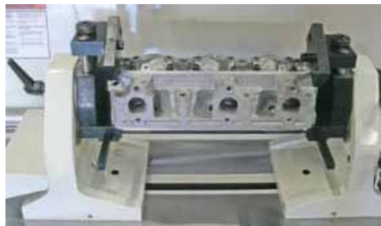
Difficult, Angle and Canted heads like GM 2.0L are easily clamped and Rolled 360 Degrees.
