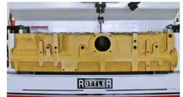
Cat 3406E cylinder head in large diesel head fixture.
