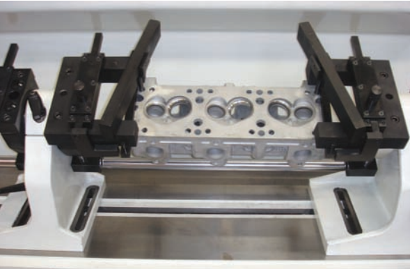
Two piece frame kit allows mounting of overhead camshaft and difficult to mount cylinder heads.
