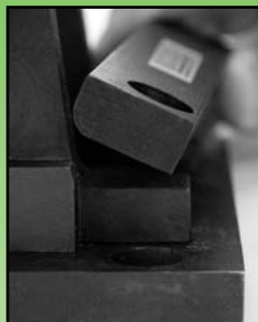
Lock the fixture to your mill bed using your standard T-Bolts (not included)
