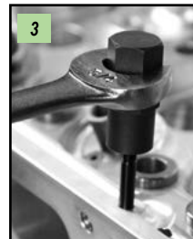
3 - Use a standard ¾" wrench or socket to tighten stud into place. Each installer is fitted with a steel ball inside to prevent over-tightening.
