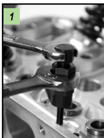
1 - Place the remover over the stud to be removed. Using 2 wrenches, back the stud out of the head.
