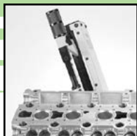
Pneumatic Head: Adjustable to 25° in either direction for canted valves
