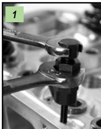
1 - Insert stud into correct size installer.
