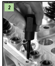
2 - Hand set the stud into the cylinder head
